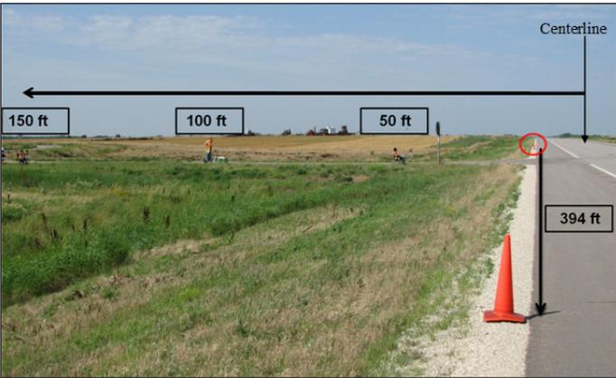
**External Noise - Set up of the Experiment**
